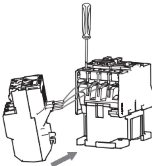
**Figure 6 Assembly drawing of thermal relay and contactor**
