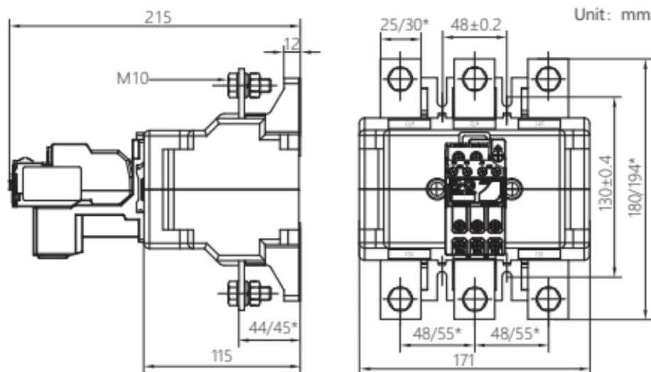
Note: Dimensions marked with "\*" means specifications for 400A and below/
