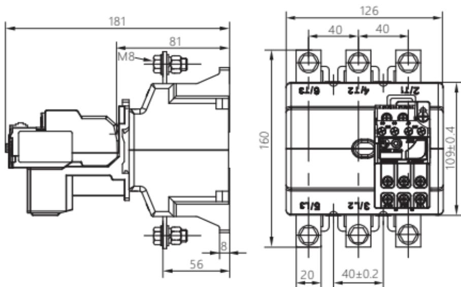
**Figure 4 Overall dimensions of NR2-200**
