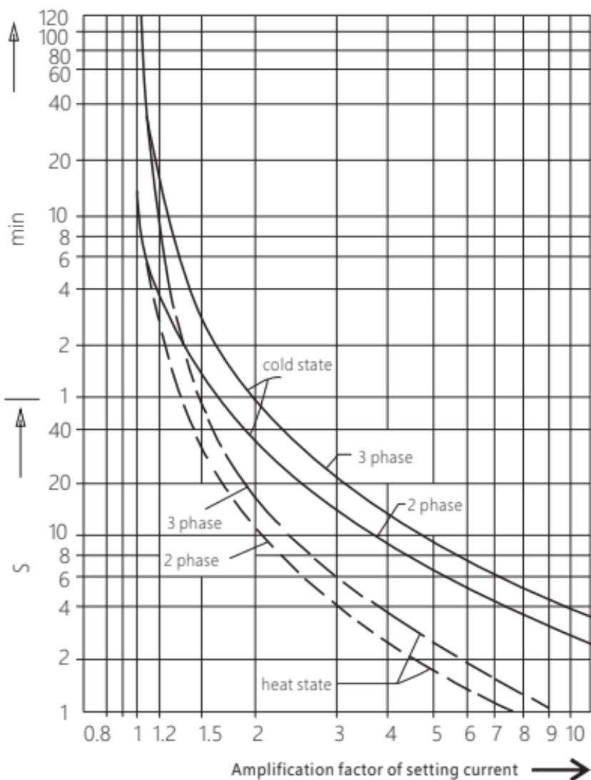
**Figure 1 Thermal relay operation time – current characteristic curve**
