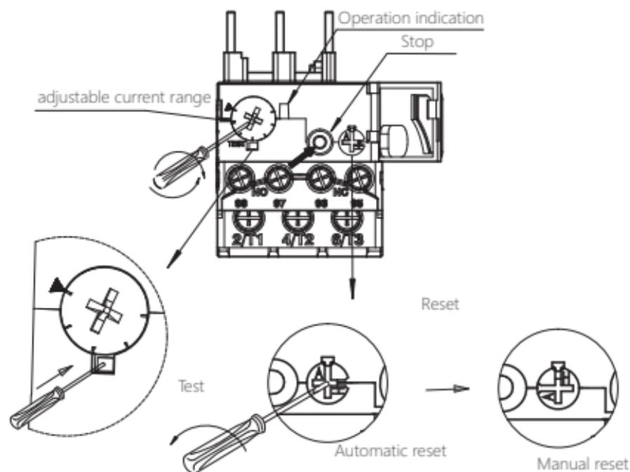
**Figure 7 Operation diagram**
